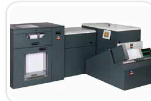
Bourg Sheet Feeder BSF working In-Line with a Watkiss PowerSquare™ 224 Booklet Maker
