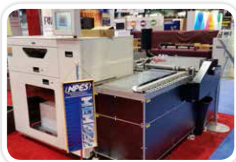
Bourg Sheet Feeder BSF working In-Line with a Rollem JetSlit card slitter
